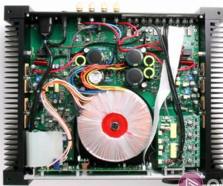
This means that the Aethos takes the same amp circuit and it sees a small rise in headline power output from 105 watts to 125 watts but the changes behind that number are more significant. The number of output devices has doubled (from two to four) and with this comes the means to completely double up the output stage. The result of this is not simply that there is more power but the ability to drive more complex and demanding loads at the same time.
