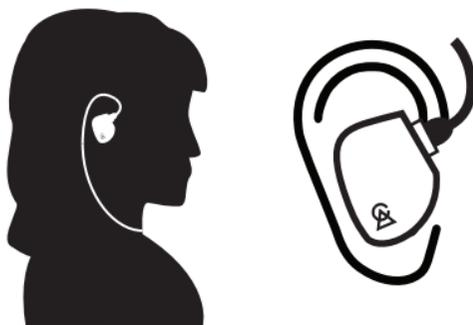
INSERT SOLARIS 2020 INTO YOUR EAR WITH THE CABLE EXITING FORWARD ALLOWING IT TO WRAP EASILY ABOVE AND BEHIND YOUR EAR. THE EARPHONES ARE 'HANDED' AND FIT EITHER YOUR LEFT OR RIGHT EAR. EACH EARPHONE HAS "LEFT" OR "RIGHT" MACHINED INTO THE TOP TO INDICATE THE SIDE.
