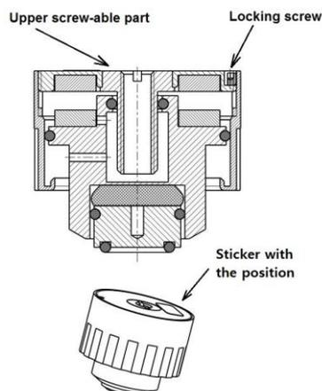
To adjust the feet, turn the small locking screw placed in the upper part of the feet about 180 degrees. Then screw the upper part by the screwdriver down to make the feet stronger.
