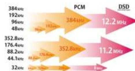
RDOT, which applies an analogous interpolation method using fluency logic, is a technology that was developed to enable the playback of the frequencies higher than 20kHz that are lost by the 44.1kHz/16-bit CD format. Based on the information read from the CD, analogous data is generated between the waveform samples. As a result, data above 20kHz is also generated. RDOT-NEO doesn't just work for PCM upconversion, it also enables conversion to the DSD format.
